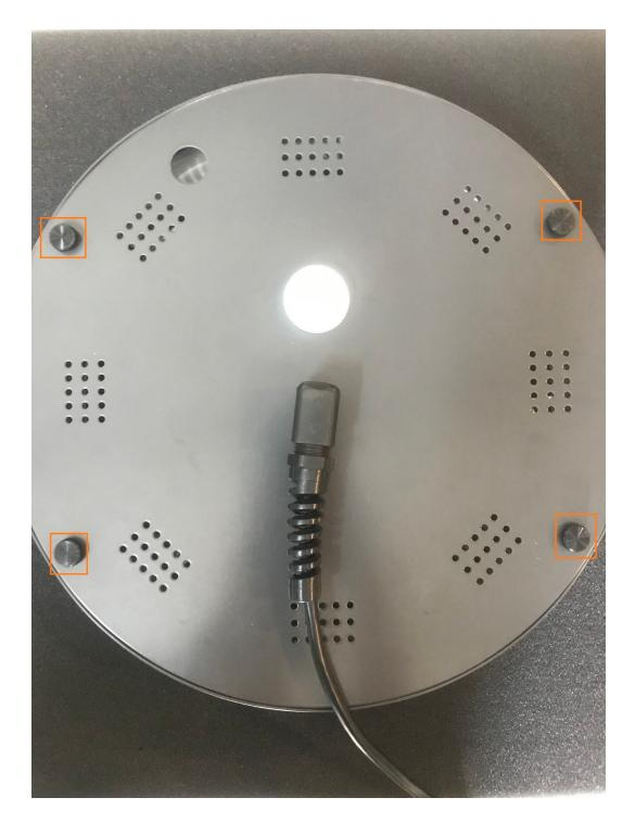
4. Pull cover aside. Remove 4 wing nuts and place iPad inside, ensuring iPad orientation is correct. Plug iPad charger into available outlet inside unit. Plug lightning cable into iPad. **Power on iPad now.** Bundle wiring neatly. Replace wing nuts and back cover thumb screws.
