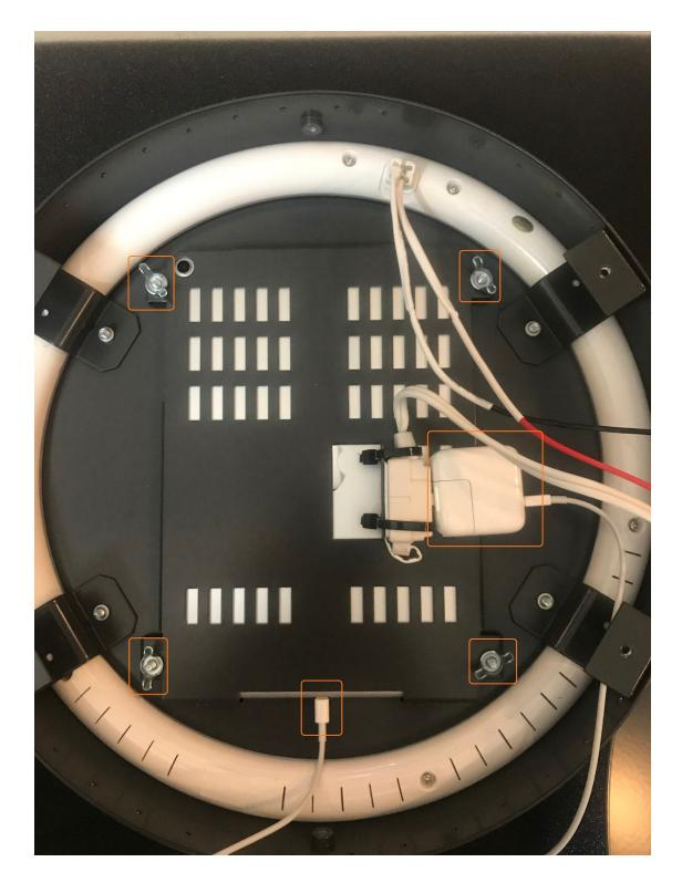
5. Mount half-circle bracket to the top of the unit using single thumb screw
