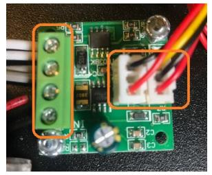
Check that connections are secure on the clear junction clips shown below. The orange clips on the opposite side can be pulled up to reseat the wires
