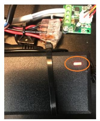
If the LED light does not come on, check that the connection below is firmly seated. Once firmly secured, you should see the LED light come on. If the LED does NOT come on, you likely have a faulty power supply. Reach out to our support team.
